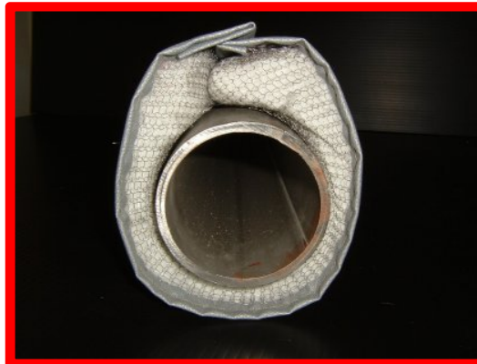
Needed insulation (fiberglass or silica) between outer layer of silicone or aluminized fabric and inner layer of stainless steel mesh.
